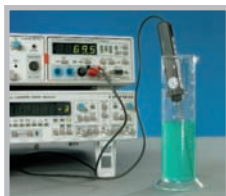
Temperature measurement HZ812 in combination with HM8012
